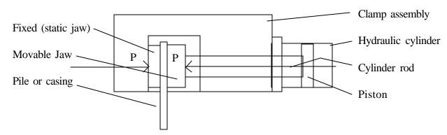
The clamping force "P" generated by the cylinder is counteracted by an equal and opposing force "P" (Static).
